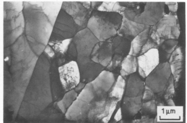
Figure 10 Substructure of type 18-2 hot rolled at 1050°C and quenched.
