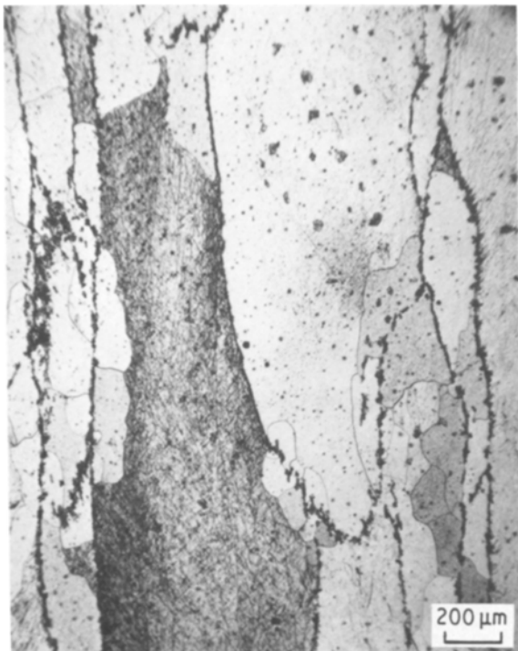
Figure 13 Grain-boundary nucleation in type 430 steel.
